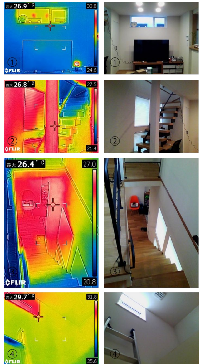
Fig. 5 Thermal images at points ① to ④
